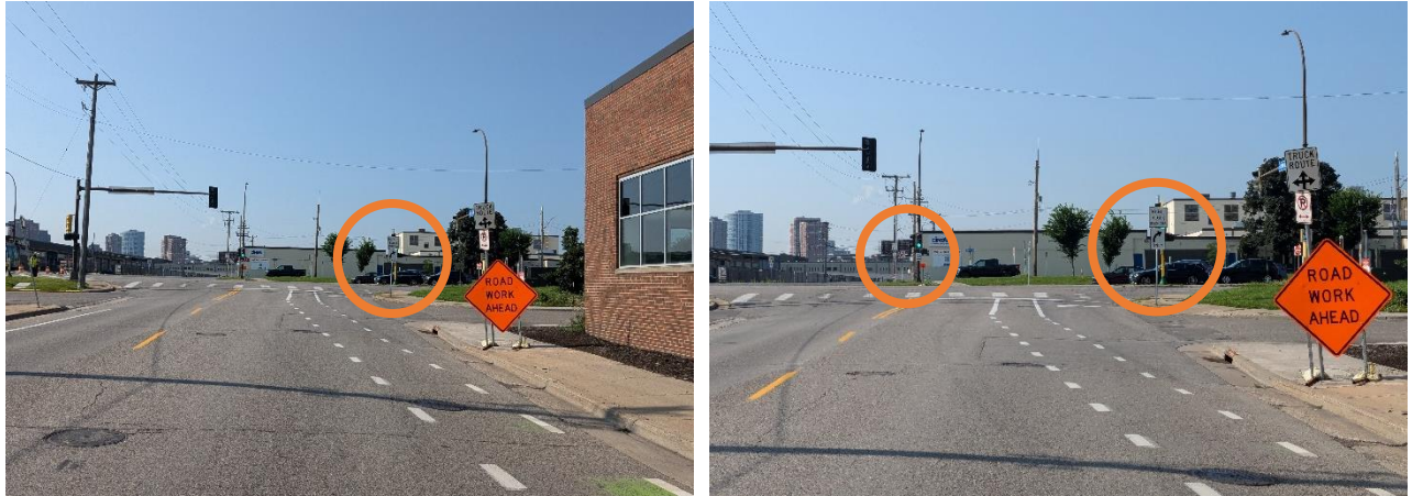
Figure 50 Driver view on approach to the intersection showing view of signals. Signal on the right has obstructed visibility.
