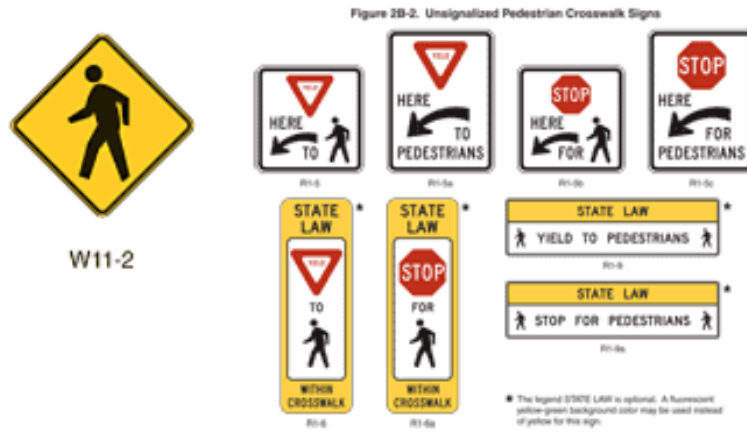
Figure 14 Examples of signs and markings used for unsignalized mid-block crossings (MUTCD 2B/3B).
